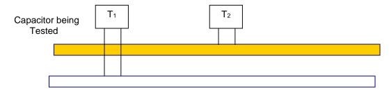
T<sub>1</sub> is the capacitor under test (Connected in the circuit)
