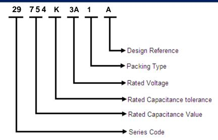
Three-digit (754) indicate rated capacitance in Pico Farad (First two digits indicate value & third digit indicates number of zeroes to be suffixed to first two digits).
