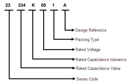
Three-digit (334) indicate rated capacitance in Pico Farad (First two digits indicate value & third digit indicates number of zeroes to be suffixed to first two digits).
