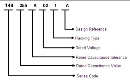
Three-digit (255) indicate rated capacitance in Pico Farad (First two digits indicate value & third digit indicates number of zeroes to be suffixed to first two digits).
