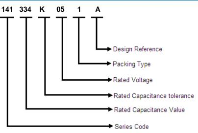
Three-digit (334) indicate rated capacitance in Pico Farad (First two digits indicate value & third digit indicates number of zeroes to be suffixed to first two digits).
