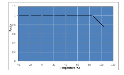
For temperature between +85°C and 105°C a decreasing factor of 1.25% per °C on the rated voltage V<sub>R</sub> has to be applied
