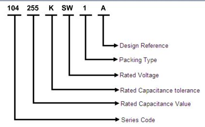
Three-digit (255) indicate rated capacitance in Pico Farad (First two digits indicate value & third digit indicates number of zeroes to be suffixed to first two digits).
