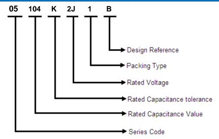
Three-digit (104) indicate rated capacitance in Pico Farad (First two digits indicate value & third digit indicates number of zeroes to be suffixed to first two digits).
