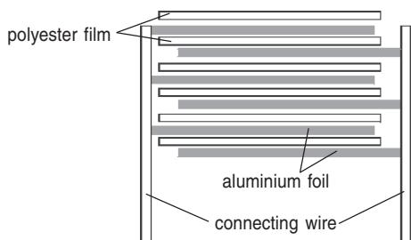
In film/foil capacitor metal foils of 5 to 6 micron thickness are used as metal electrodes.
