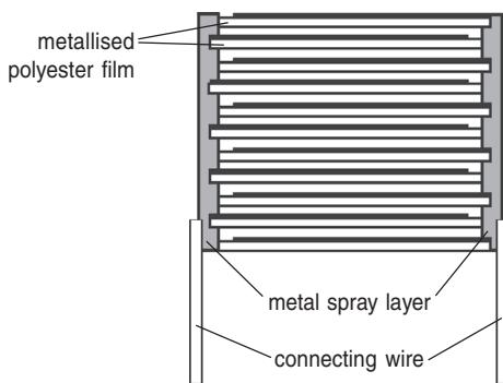
Here instead of using 6 micron thick foil, the plastic film (dielectric) is coated with either aluminium or zinc alloy material. Metal particles are vacuum deposited directly on to the plastic films. Thickness of the metallisation is approximately 30 nm. This drastic reduction in thickness of electrodes leads to the relatively smaller dimensions for metallised film capacitors.
