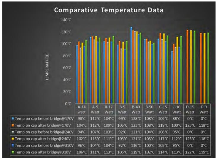
\*0°C in graph above indicates the absence of a capacitor in that position.
