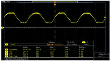
Voltage wave form for stress after the bridge
