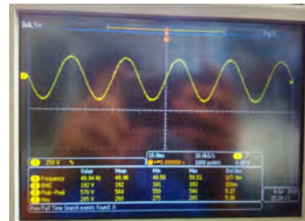
Stress across capacitor at step 1 and 300 V AC Input
