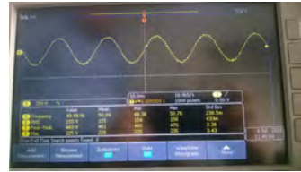
Stress across capacitor at step 1 and 230 V AC Input
