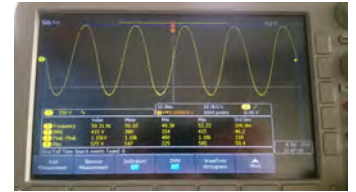
Stress across capacitor at step 5 and 230 V AC Input
